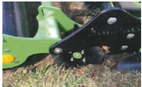
Option : edge trimming with sharpened disc
