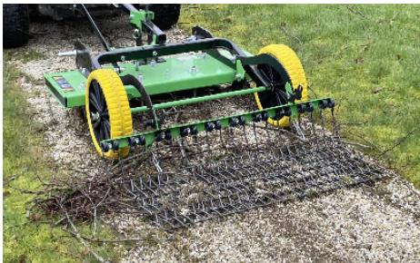
Rake, harrow and grid for clod crumbling
