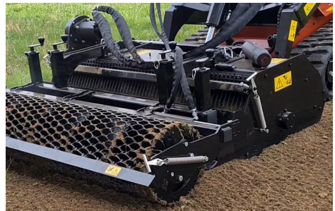
Option : Roller side adjustment device by cylinder
