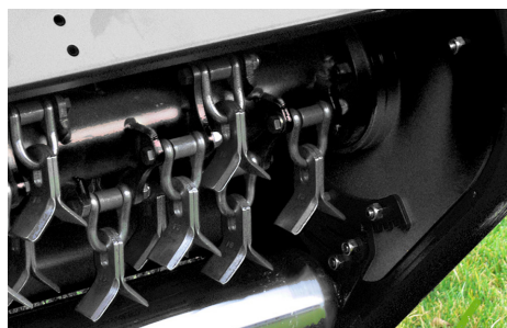
Y-shaped mounting of knives on shackles
